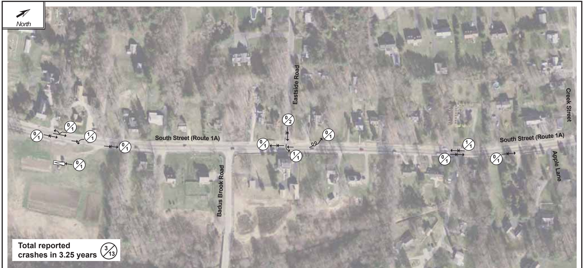
Figure H-8 Collision Diagram: Route 1A between Creek Street and Beach Street Wrentham Police Reports: January 2014 – March 2017
