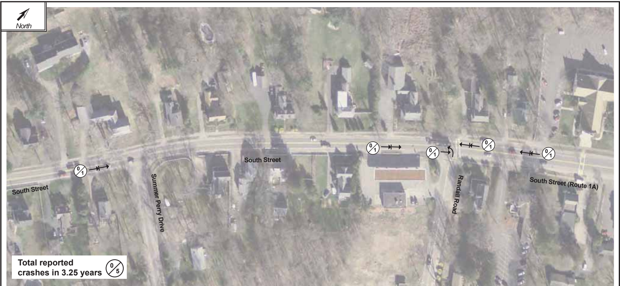
Figure H-6 Collision Diagram: Route 1A at Randall Road and at Summer Perry Drive Wrentham Police Reports: January 2014 – March 2017
