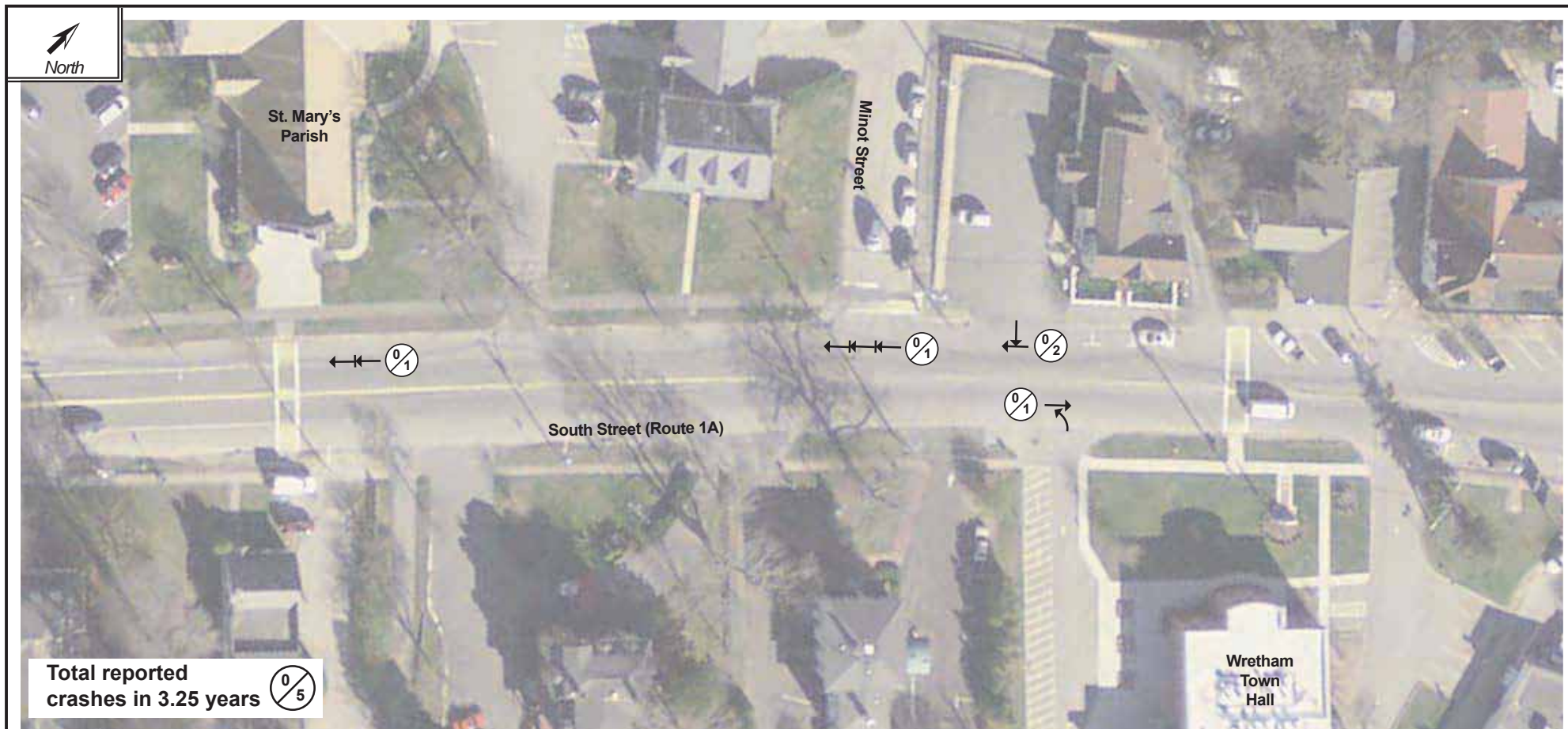
Figure H-5 Collision Diagram: Route 1A in the Vicinity of Wrentham Town Hall Wrentham Police Reports: January 2014 – March 2017
