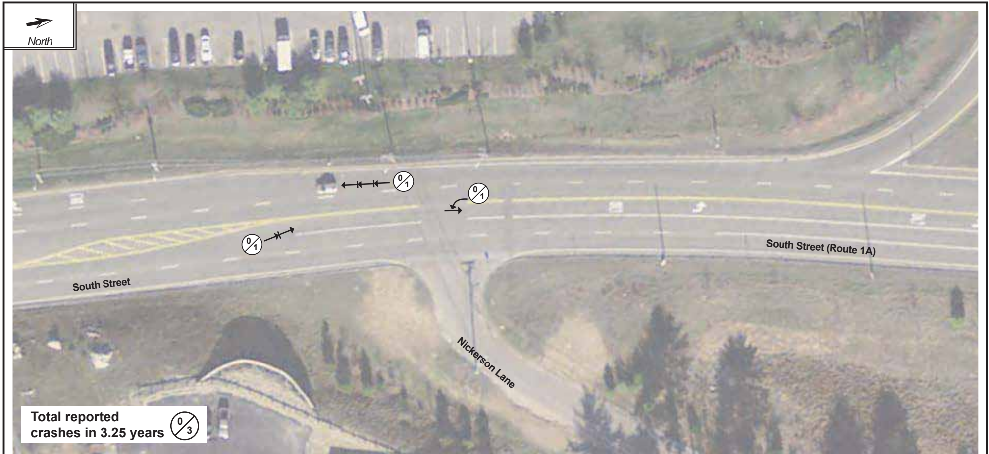
Figure H-16 Collision Diagram: Route 1A at Nickerson Lane Wrentham Police Reports: January 2014 – March 2017
