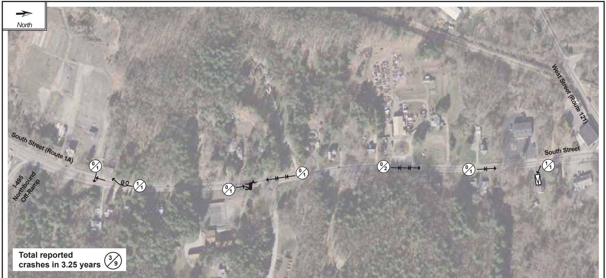
Figure H-12 Collision Diagram: Route 1A between Route 121 and I-495 Wrentham Police Reports: January 2014 – March 2017
